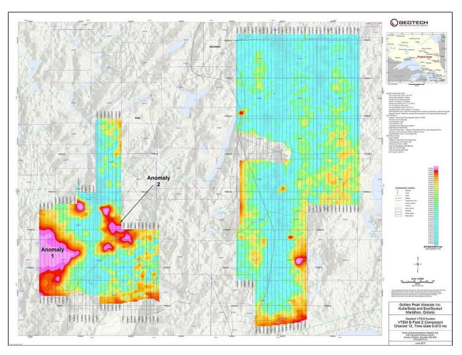
FIGURE 2.0 Heikki Project VTEM TM B Field Z Component Conductive Anomalies
